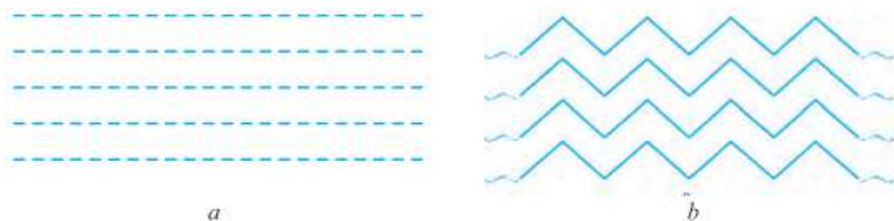
2-rasm. Parallel va zig-zak baxya qator tikish
